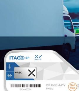
ITAG<sup>®</sup>4 series data loggers are developed to monitor and capture temperature or humidity excursions in pharmaceutical, biological and clinical trial supply chains. With TempSen's advanced measurement technology, user could easily have a reliable monitoring results accurately reflecting the supply chain environmental conditions.
